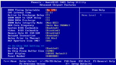
**NOTE:** This "Advanced Chipset Features" option controls the configuration of the board's chipset, this page is developed by Chipset independent, for control chipset register setting and fine tune system performance. It is strongly recommended only technical users make changes to the default settings.
